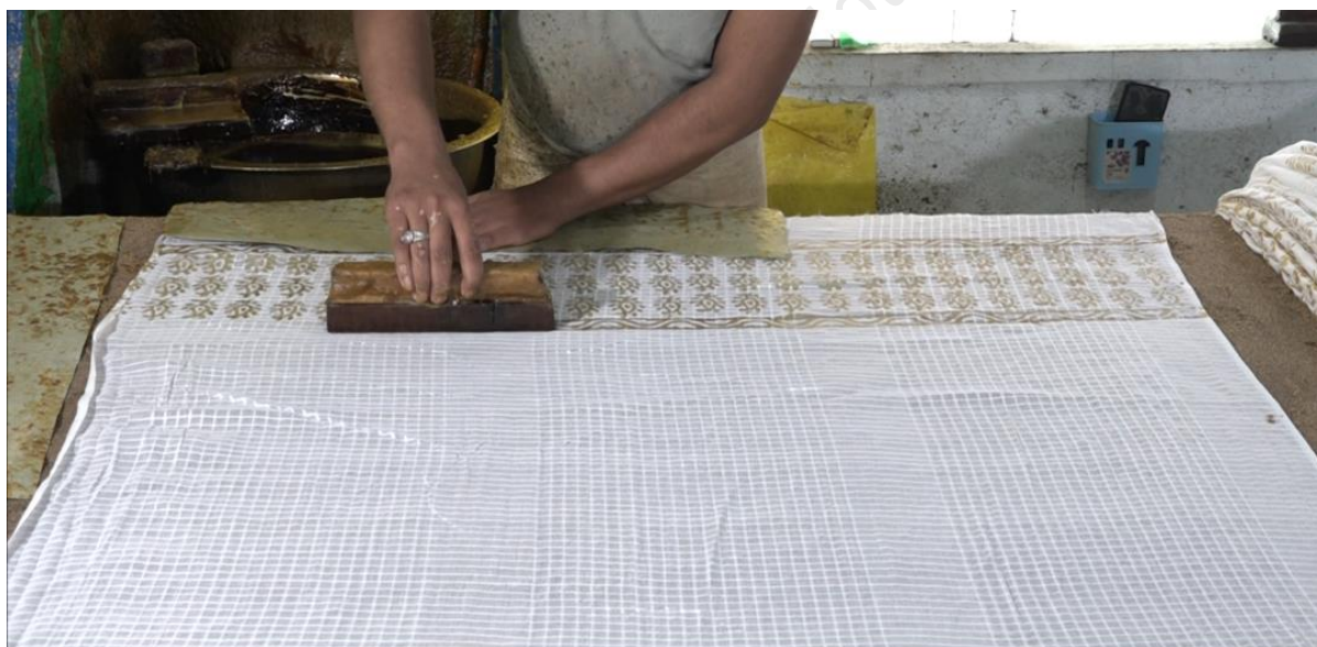
Fig. 3.27: Skilled artisans ensure print precision through alignment, clean blocks and quality dye preparation
